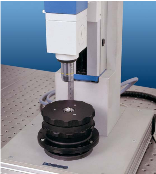
Centration and MTF Measurement with OPTOMATIC MICRO
