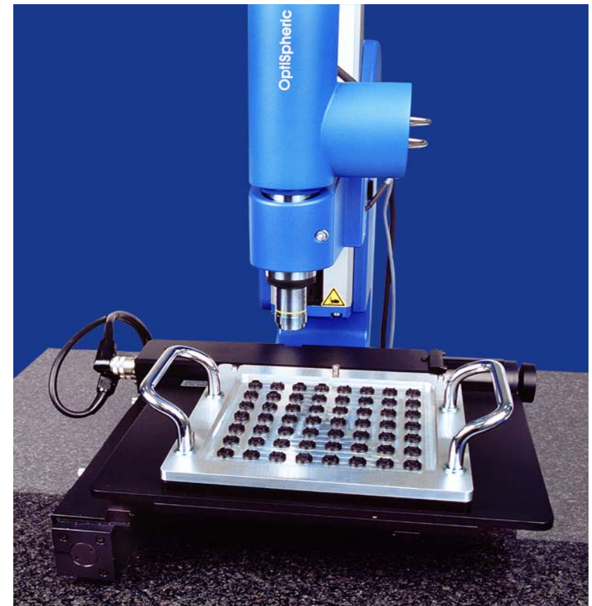
OptiSpheric IOL Tray system for volume testing in production
